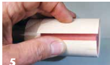
5 Use softened maple veneer for the middle layer. Trim the size to give an exact fit around the core cylinder.
