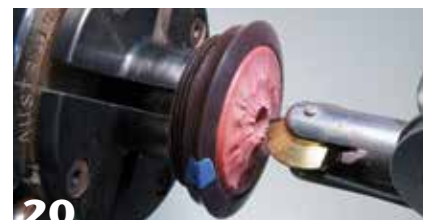
20 Pattern the lid of the box being careful to align the pattern with the side of the box (note the blue tape).
