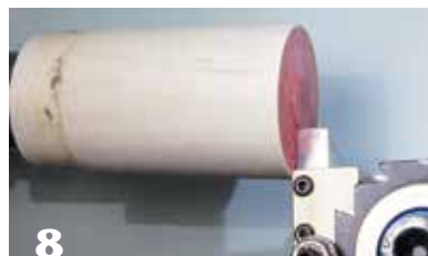
8 Trim the excess off the end of the cylinder.
