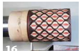
16 Part off with the cut-off tool and catch the cylinder with your finger.
