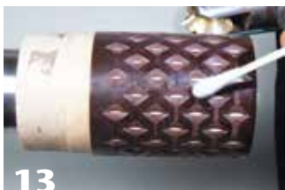
13 On the rose engine, start to cut the pattern so it barely goes through the outer layer and apply CA glue with a cotton swab.
