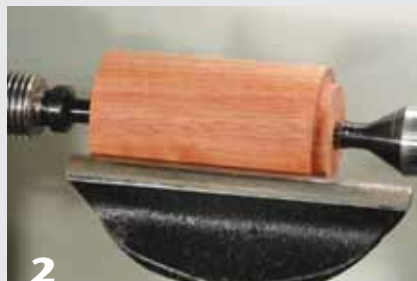
2 Turn the block to 2.25" (57 mm) in diameter and turn a tenon on one end for mounting in a four-jaw chuck.
