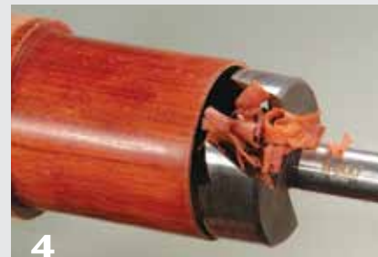
4 Drill out the center with a 1\frac{7}{8}" (48 mm) Forstner bit.
