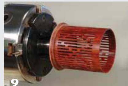
9 Glue the pierced cylinder to the base, and turn the edge of the base to form a pleasing curve.
