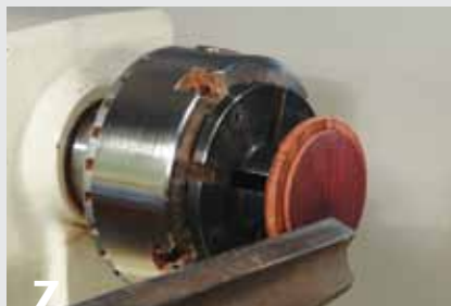
7 Turn a 0.1" (2.5 mm) tenon on the top of the base. This tenon will form a snug fit with the turned and pierced cylinder.
