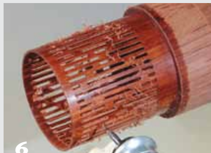
6 After piercing, clean-up work with fine sandpaper is necessary.
