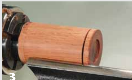
3 Clean up the cylinder's face and cut a recess 0.1" (2.5 mm) deep and 1.25" (32 mm) in diameter, part off the base, and set it aside.
