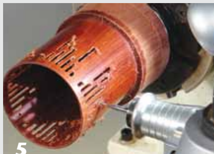
5 Pierce the cylinder using a ¼" (1.6 mm) end mill and the cutter mounted on a compound or slide rest.
