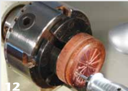
12 When piercing the lid, go all the way through the top and into the jam chuck.
