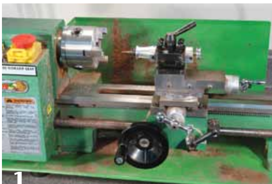
1 A Foredom handpiece is mounted on the compound tool-rest of a mini metal lathe.
