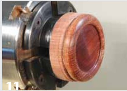
11 Make a jam-fit chuck for the lid, then turn a recess 0.075" (1.9 mm) deep and to a diameter of 1.6" (41 mm).
