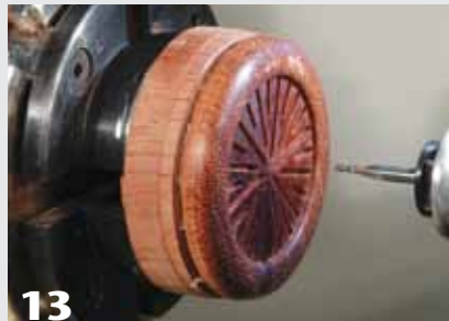
13 After all the cuts are made, clean up the rough edges with fine sandpaper.
