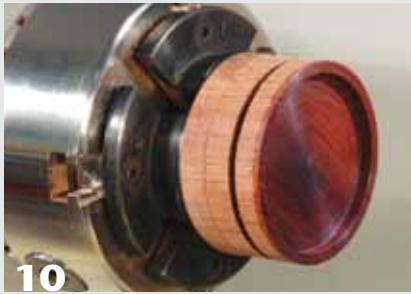
10 The inside of the lid is recessed 0.15" (3.8 mm) at a diameter that will form a snug fit with the pierced cylinder.
