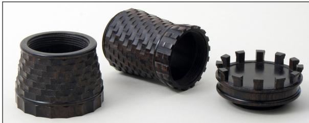
The “brickwork” decoration is done with a 1/8” diameter cutter that has a sharpened flat end. It’s mounted in a “universal cutting frame” that is rotated so the cutting motion is vertical. At each index point, the cutter is moved into the wood by a fixed distance. Each successive layer of “brickwork” is shifted by 1/3 of the pattern to give an attractive spiraling effect. This is difficult to do with a traditional index wheel, but it’s easy with the computer-driven stepper motor.
