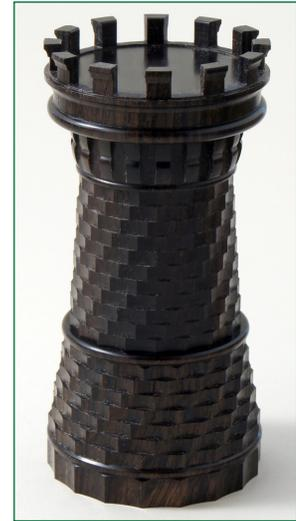
The “corbels” at the top of the centerpiece are done with a 1/8” diameter end mill mounted in a “drilling frame.” At each index point, the cutter is moved to cut a groove in the work. As with any router-like work, it’s better to take several shallow cuts rather than one single deep cut. Likewise, the top of the turret is cut with a 1/4” diameter end mill mounted in a “drilling frame.”
