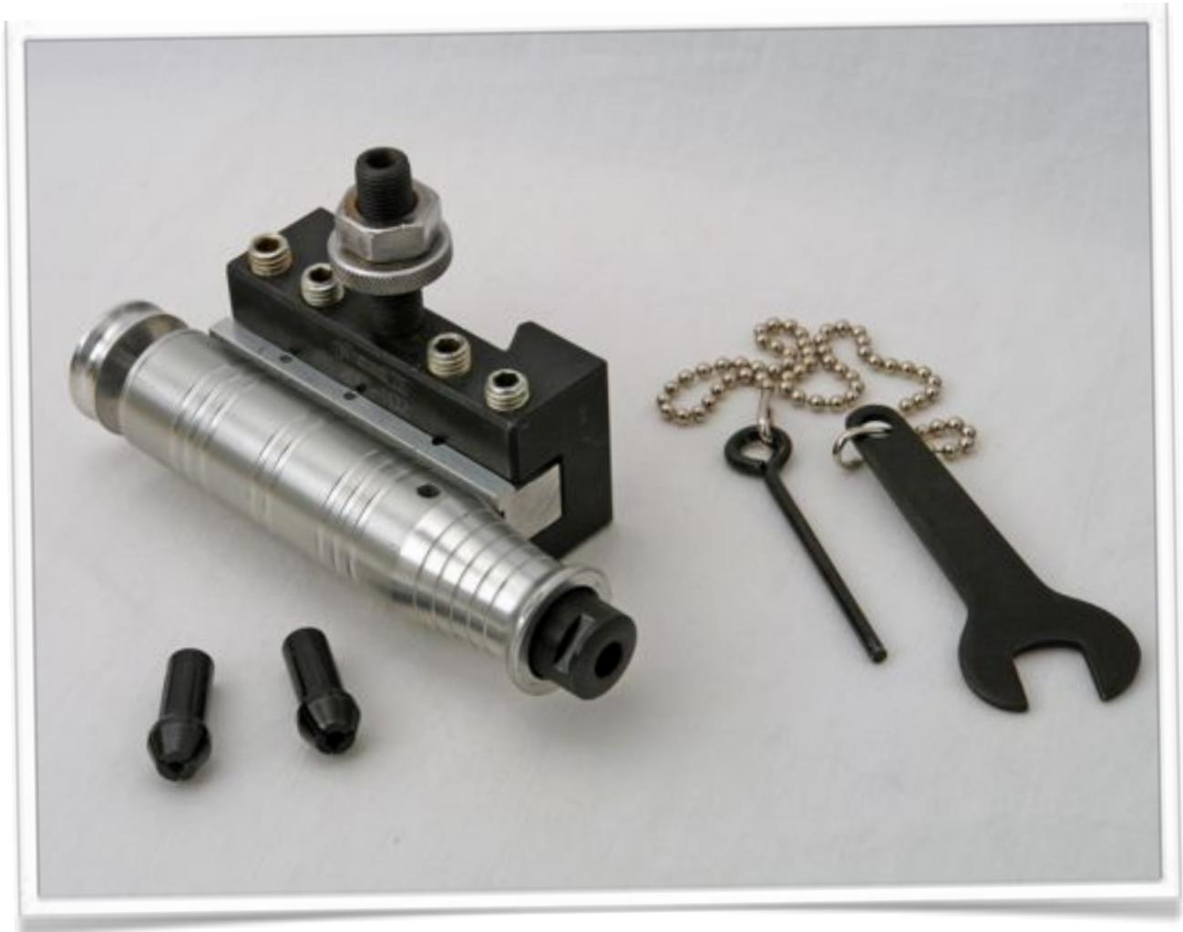
This article describes the construction of a drill frame (which can be used for an eccentric cutter) made from a Freedom hand-piece.
