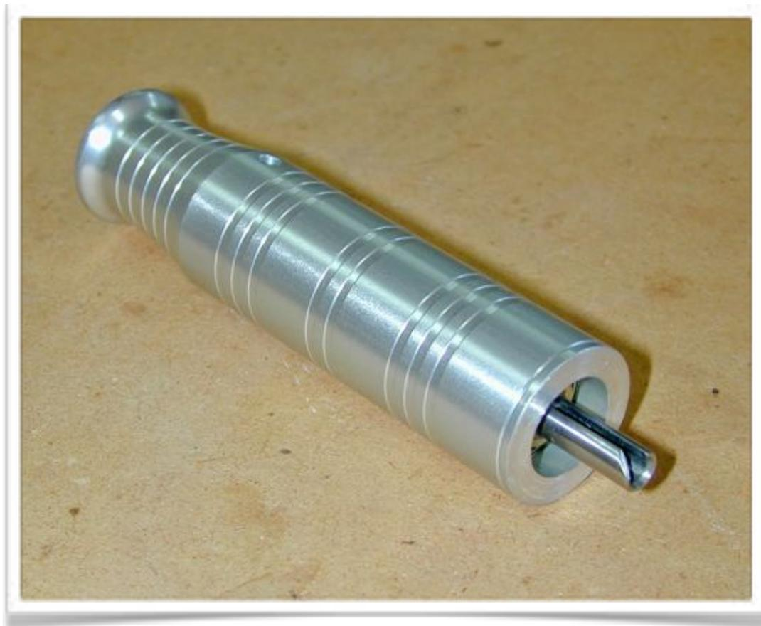
The exposed shaft is 1/4" diameter and hollow with a slot to fit the end of the Foredom flexible shaft. I made a 1" diameter pulley to press fit onto the end of the shaft. The hole in the pulley is slightly smaller than the shaft to allow for a tight press fit. (I used a "D" drill, 0.0246").
