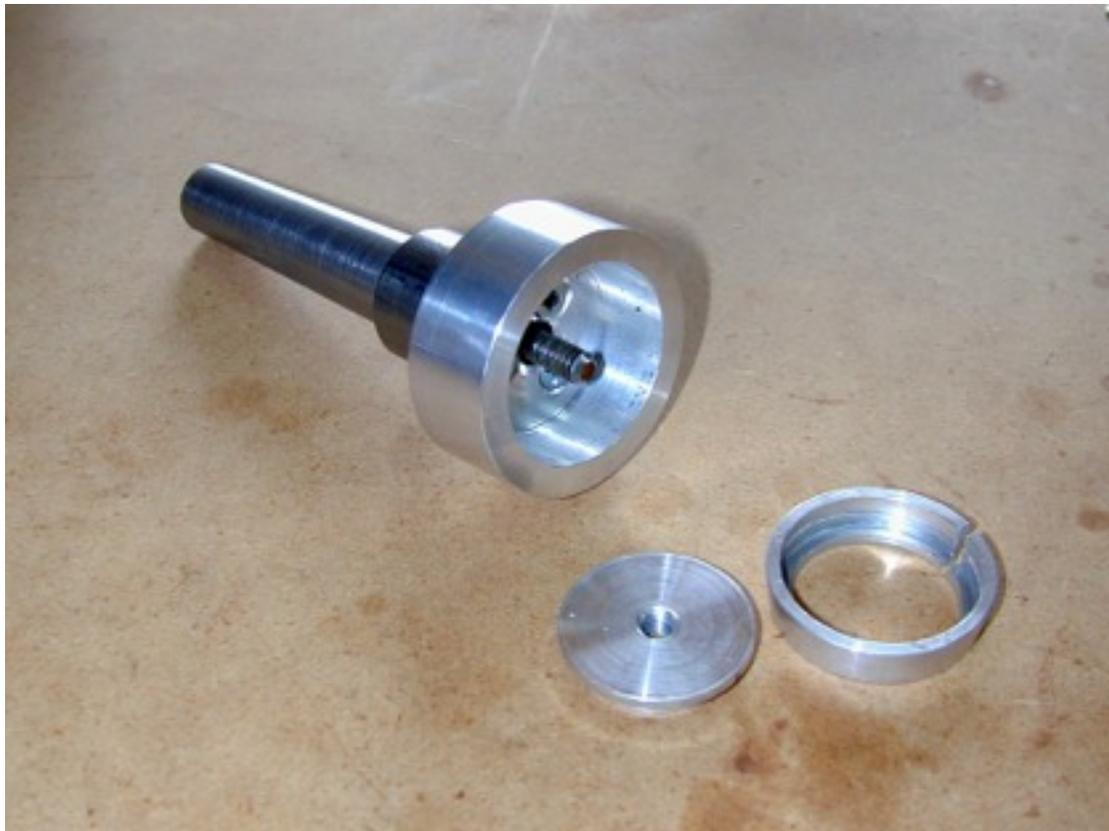
I made the interior of the ring 1.3" diameter which is the smallest tenon that my Vicmarc VM100 chuck can grab. This size also works well on my metal lathes (which I use for wood). I tested the split collet concept by attaching it to a MT2 taper. It seems to hold the work well enough (although for roughing out and hollowing I would still use my Vicmarc chuck).
