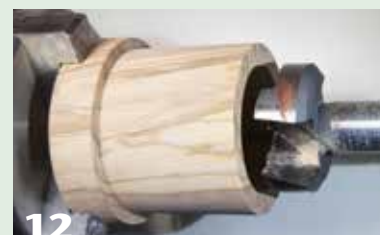
12 Drill out the bulk of the material with a Forstner drill bit.
