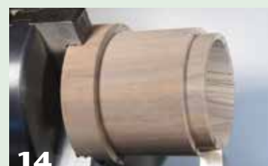
14 Cut a tenon for the lid by taking multiple cuts to the final dimension.
