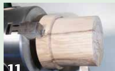
11 Make multiple cuts to reduce the outer diameter of the body of the box.
