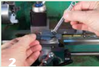
2 Adjust the jibs on the dovetail slides with an Allen wrench and then gently tighten the locking nut.
