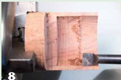
8 Cut-away view shows the use of a boring bar inside a cylinder moving from right to left.
