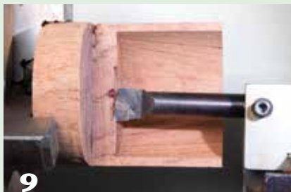
9 Cut-away view shows the use of a boring bar on the bottom of a cylindrical hole.
