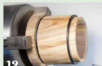
18 Part off the cylinder with the cut-off tool.
