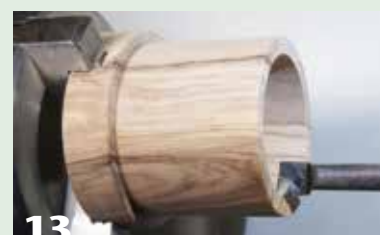
13 Make multiple cuts with a boring bar to enlarge the inside of the cylinder to its final dimension.
