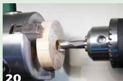
20 Make a recess in the lid with a two-fluted end mill.
