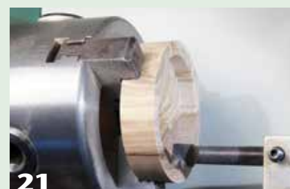
21 Enlarge the recess in the lid with a boring bar to provide a snug fit on the tenon on the body of the box.
