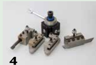
4 A quick-change tool post with an assortment of tool holders and cutters.
