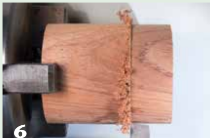
6 Cut on the outside of a cylinder moving from right to left—note that the end of the tool is not scraping flat.
