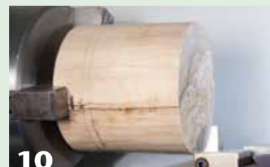
10 Make a clean and square cut on the end of the body of the box.
