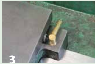
3 A modification to the carriage saddle allows me to lock the carriage with a brass screw in a drilled and tapped hole.
