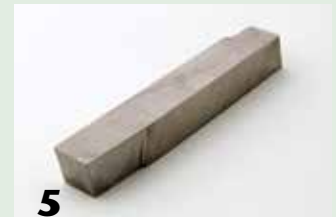
5 The basic cutter is a 3/8" square HSS tool blank sharpened like a scraper on the end and one side.
