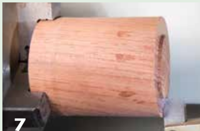
7 Cut on the end of a cylinder—note the tool is at a slight angle and the side is not scraping flat.
