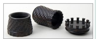
The "brickwork" decoration is done with a 1/8" diameter cutter that has a sharpened flat end. It's mounted in a "universal cutting frame" that is rotated so the cutting motion is vertical. At each index point, the cutter is moved into the wood by a fixed distance. Each successive layer of "brickwork" is shifted by 1/3 of the pattern to give an attractive spiraling effect. This is difficult to do with a traditional index wheel, but it's easy with
