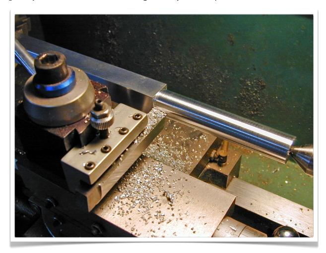
Drill the holes for the spring pins and screw as describe in the HCF construction notes. Then drill and ream the hole at the end of the arms for the bearings as described in the HCF notes, and make the two pulleys that will mount on the sides of the frame.
